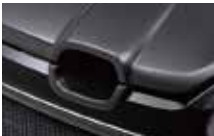
AIR INTAKE DUCT
